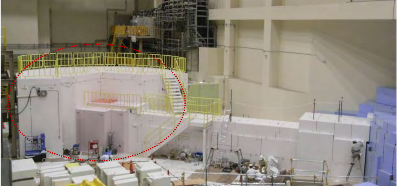
Fig.6 Sckematic veiw of the BL14 (dot circle indicate the spectrometer sheilding which inside wall is covered by boron-enriched mortar)
